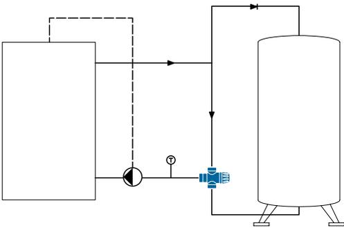
MIXING IN THE STORAGE LOADING CIRCUIT
