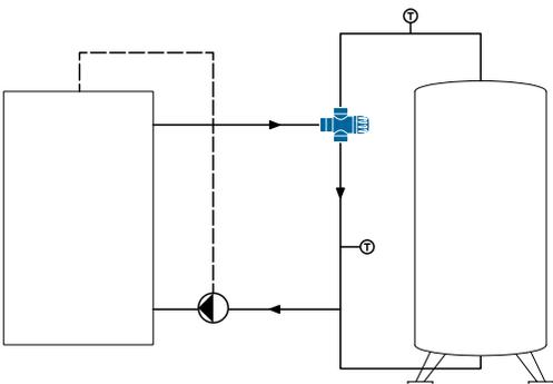
CIRCULATING IN THE STORAGE LOADING CIRCUIT
