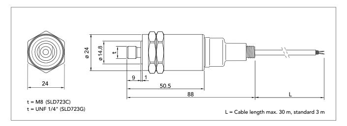
The 4-20 mA vibration transmitters are piezo-electric accelerometers of compression type and provide a 4-20 mA output signal proportional to the true RMS value of vibration velocity. The transmitters can be connected to common process control systems (PLC, DCS). The electrical signal is isolated from the transmitter housing. The transmitters operates by using power from a standard 4-20 mA loop.
