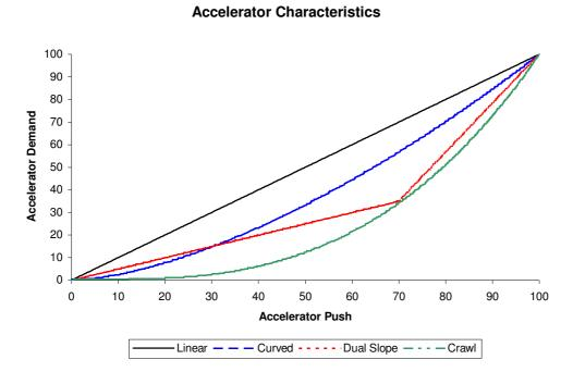
**Figure 9: Accelerator Characteristics**
