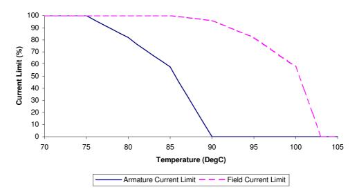
Figure 10: Armature Thermal Cutback Characteristic
