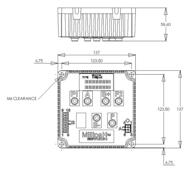
Figure 1: MillipaK Core Dimensions
