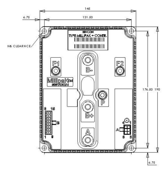
Figure 2: MillipaK HP Dimensions
