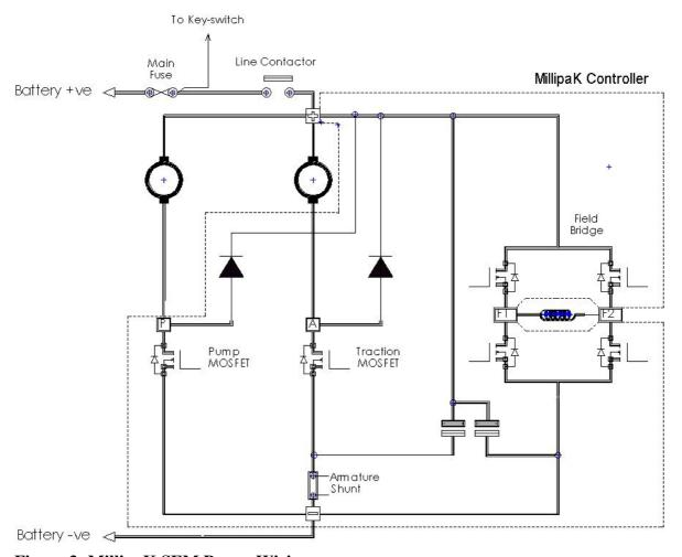
Figure 3: MillipaK SEM Power Wiring
