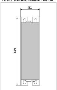
Fig. 25-5 Hole pattern for wall mounting
