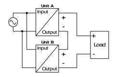
Pay attention that leakage current, EMI, inrush current, harmonics will increase when using multiple devices.
