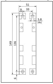
Fig. 25-6 Wall/panel mounting, side view
