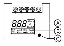
The device has an integrated Power Supply Condition Display (PSCD). It shows all the different power supply condition values on the front of the PSU for condition monitoring and easy analysis of power errors. When switched on, all LED segments of the PSCD light up for 2 seconds to indicate the full functionality of the display. At the next turn-on procedure, the PSCD shows the menu of the last turn-off sequence.
