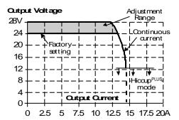
Fig. 6-3 Output voltage in "parallel use" mode, typ.
