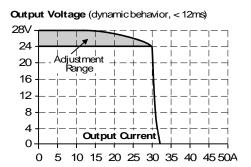
Fig. 6-4 Short-circuit on output, Hiccup<sup>PLUS</sup> mode, typ.
