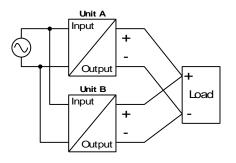
Energize all units at the same time. It also might be necessary to cycle the input power (turn-off for at least five seconds), if the output was in overload or short circuits and the required output current is higher than the current of one unit.
