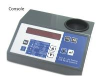
The console is the central control unit for the Oil Analysis range.
