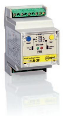
The **ELR-3F**, maintains all the basic characteristics of the ELR-3C type relay, with its reduced dimensions even. It is the most simple of a series of relays, built in a modular enclosure, according with DIN 43880 Standard, with a three modules width (module base 17.5 mm)
